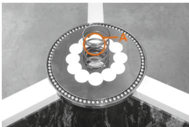
Put one of the both plastic guides with thicker socket ahead into the central hole and insert the **COMPRESSION SPRING (A)**.
