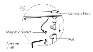
(5) Magnet must be attached to the rod.
