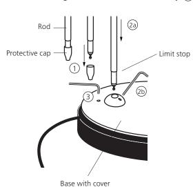
(3) The ball joint can be readjusted here.
