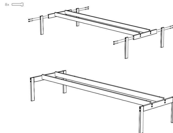
3. Align the holes in the legs with the pre-drilled holes in the cabinets and insert the included screws.
