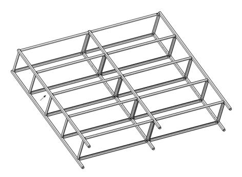
Re-install the last corner profile (only holes on one side).
