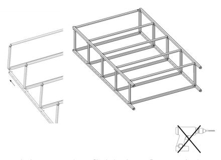
Insert 10 screws both corner extension profiles by hand power. Do not use a hex key or power tool. Do not tighten the screws fully. Install the two extension profiles (with holes on both sides) by sliding them onto the frame.
