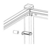
Insert the screw and tighten it fully to secure the rack to the wall.
