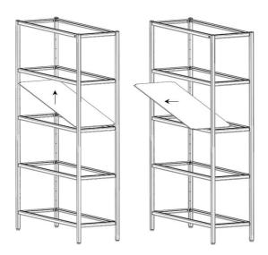
Remove all ceramic plates from the rack. It is advised to be two persons to lift and remove the ceramic plates. Lift the ceramic plates in an angled position and remove them from the frame. Avoid bumping the plates against the frame.
