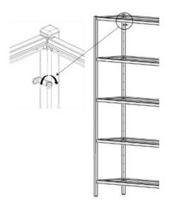
Install the wall mount in the free hole at the top of the rack facing the wall. Install the wall mount at the same height as the two wall mounts already installed.
