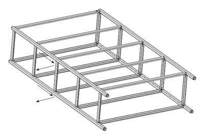
Remove the two corner profiles on the left. Remove all screws on the corner profile and slide it down the frame to remove it.
