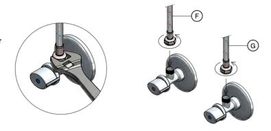
Turn on the water supply, check for leaks and retighten if needed. Once leak free, your mixer tap is ready for use.
