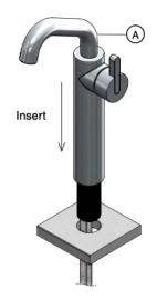
Slide the NBR washer  $\odot$  and stainless steel washer  $\odot$  onto the threaded sleeve  $\odot$ , then screw on the fixing nut  $\odot$  while holding the tap in place.
