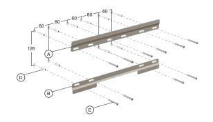
Slide the shelf  $\bigcirc$  onto the mounting bracket  $\bigcirc$  and  $\bigcirc$  .
