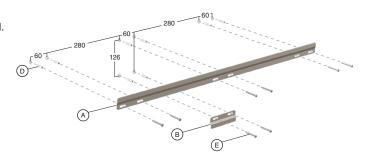
Slide the shelf © onto the mounting bracket A and B.
