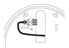
Plug the cable from the ceiling outlet into the terminal clamp and secure it with the strain relief.
