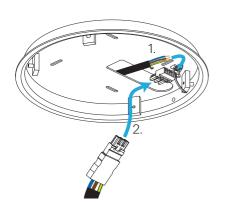
Connect the WAGO terminal clamp from the ceiling fixture to the ceiling fixture cover.
