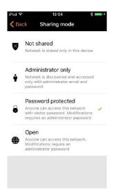
Note that Evolution networks offer three levels of user access: user, manager and administrator. Users can control the lights, Managers can configure the network but not change sharing or security settings. Also adding new devices to the network requires Administrator access to the network
