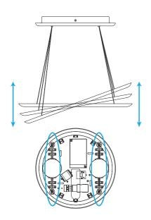
Note the alignment of the ceiling fixture during installation. The luminaire can be tilted over one axis. Only the two wires belonging together can only be adjusted at the same time.
