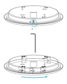
Loosen the countersunk screws and unscrew the ceiling fixture cover from the bayonet holder and remove the ceiling fixture cover.
